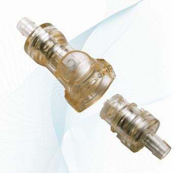
HFC39 Series sterile disconnect couplings prevent external organisms from entering into the media flow path upon disconnection. Automatic shutoff valves close off the flow path aseptically protecting valuable media while also eliminating the need for pinch clamps and tube welders. The easy-to-use thumb latch design provides a secure, leak-free connection and enables one-hand disconnects.
