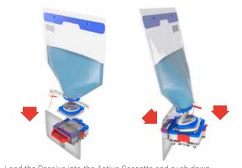
Load the Passive into the Active Cassette and push down at the rear
