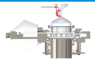
Contact surfaces of the passive and active system exposed to UV-C light
