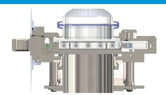
Underside of the passive and upper face of the active slider exposed to UV-C light
