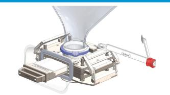
Remove clamp / gripper at the neck of the chargebag to transfer product through the system
