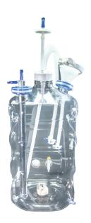
Mixed4Sure™ Bottom Mount Pro is an aseptic, closed-system mixing platform that offers low shear and vigorous mixing. Available in several volumes and custom configurations, enabling it to be used in a variety of mixing steps. The M4SB Pro integrates a Heating/Cooling Finger and pH and conductivity sensors.
