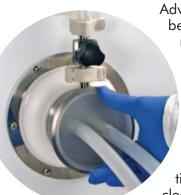
AdvantaPass permits the aseptic transfer of fluids between the walls of pharmaceutical and biopharm manufacturing suites. It's the first system of its kind to offer complete isolation between different classes of clean rooms when transferring multiple lines of fluid through a single wall portal.
