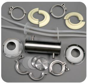
AdvantaPass® uses 316L stainless steel components such as portals, end caps and hygienic union clamps to form a secure barrier, while it incorporates Single-Use tubing, seals and isolator assemblies for fluid transfer processes. AdvantaPass is offered in standard sizes up to 6" diameter with larger dimensions available on request.
