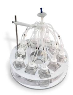
One2Fill™ (Simultaneous Fill) is a range of standard manifolds with bottles for aliquoting or sampling in a variety of upstream and downstream applications, including media or buffer preparation, and other filling applications.
